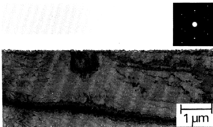
Figure 20. Transmission electron micrograph of an ultramicrotomed section of the thermal oxide film grown on the (111) face of copper which has been oxidized in purified oxygen at 178 °C for 10 min.
