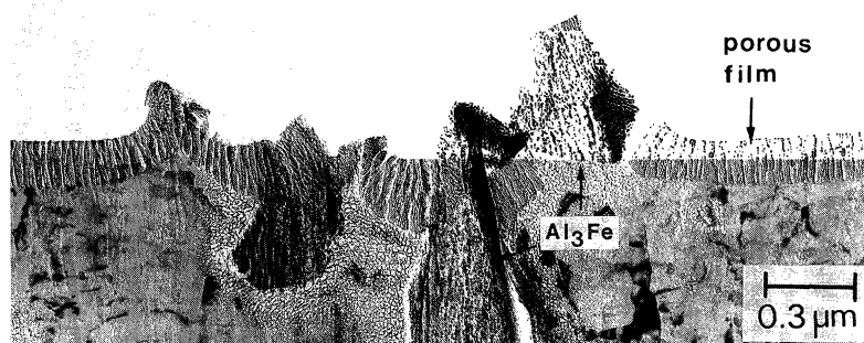
Figure 14. Transmission electron micrograph on an ultramicrotomed section of the porous oxide film grown in an Al–1.5 wt% Fe alloy at a constant current density of 5 \text{ mA cm}^{-2} in 2.4 M sulphuric acid at 25^\circ\text{C} for 2 min.
