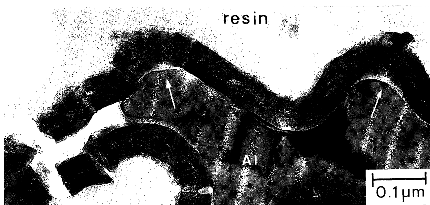
Figure 13. Transmission electron micrograph of an ultramicrotomed section of the barrier oxide film, formed on an AC etched aluminium foil.
