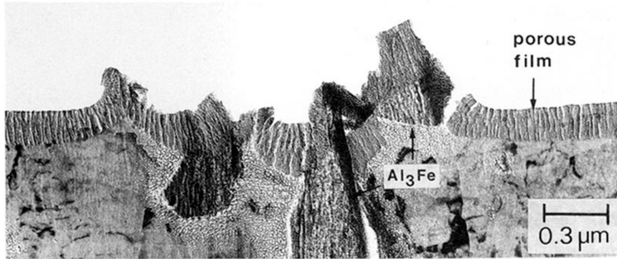
Figure 14. Transmission electron micrograph on an ultramicrotomed section of the porous oxide film grown in an Al–1.5 wt% Fe alloy at a constant current density of 5 \text{ mA cm}^{-2} in 2.4 M sulphuric acid at 25^\circ \text{C} for 2 min.
